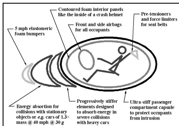
**Figure 3** Multistage energy-absorption schematic
