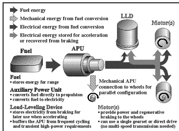
Figure 1 Series and dual-mode-parallel HEV schematic
