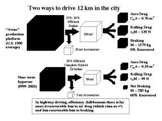
Figure 2 Early hypercars' schematic physical principles
