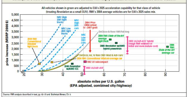
Thus the average 2025 ultralight-hybrid car would get 92 mpg, *vs.* the 2004 *Prius*'s 55, at virtually the same marginal cost, which is due to its hybrid powertrain. (*Prius*'s many buyers obviously find that cost worthwhile.) Also graphed in magenta is the steel industry's ultralight-steel *Taurus*-class car—recalculated by RMI as a ~72-mpg hybrid—that would be a worthy competitor and a conservative technological backstop to the carbon-fiber ultralight.
