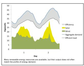
If this exact matching fails, the grid rapidly destabilizes, its components disconnect to prevent serious damage to the equipment, and the lights go out. Historically, utilities have met this exacting requirement by first measuring what they assumed was an uncontrollable demand, then tightly controlling their power plants' output to match the demand.
